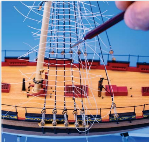
Apply watered down PVA wood glue to the ends of each ratline using a small brush.
